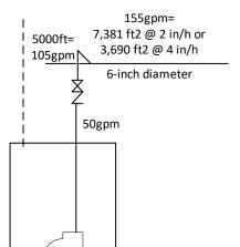
at 2 in/h rainfall, 50gpm are equivalent to 50/0.021=2381 ft<sup>2</sup> (Table D101.1)
