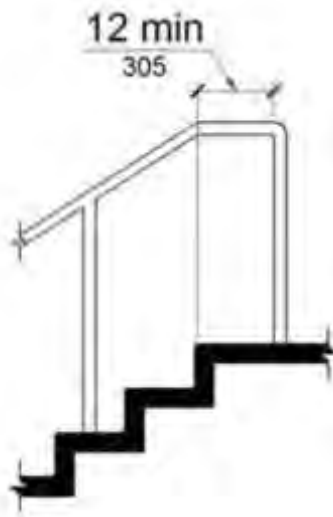
FIGURE 11B-505.10.2 TOP HANDRAIL EXTENSION AT STAIRS
