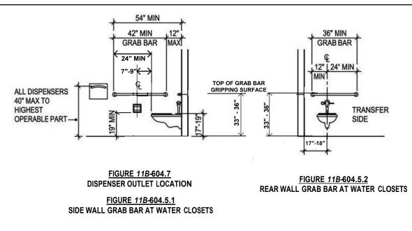
THESE DIAGRAMS ILLUSTRATE THE SPECIFIC REQUIREMENTS OF THESE REGULATIONS AND ARE INTENDED ONLY AS AN AID FOR BUILDING DESIGN AND CONSTRUCTION.
