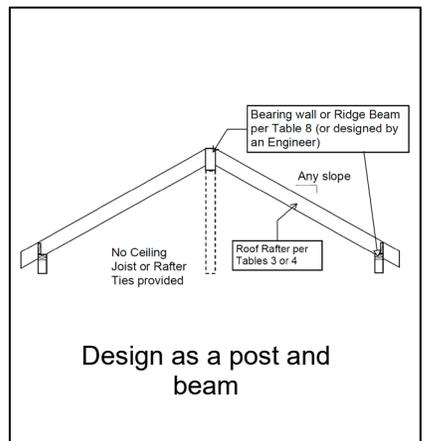
1. Rafter spans shall be measured along the horizontal projection of the rafter.
