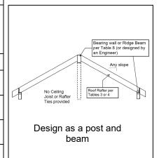
Rafter spans shall be measured along the horizontal projection of the rafter.
