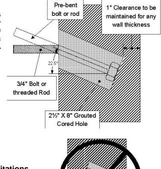
Detail E.1 – Grouted  $22\frac{1}{2}^{\circ}$  Inclined Anchor Limitations  $22\frac{1}{2}^{\circ}$  grouted anchors shall not be installed with inclination upwards or sideways.
